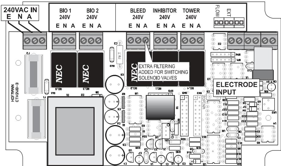
The Set point relay terminals connect to earth, neutral and switched active 240V. (240VAC is supplied to these terminals when activated by the set point.)
