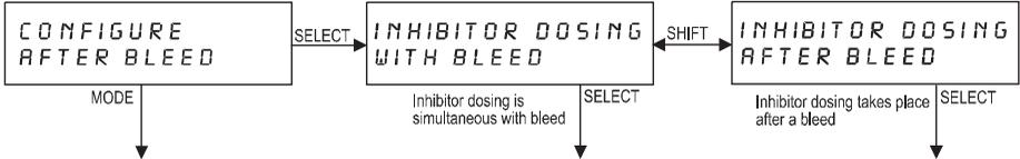
Bleed times are added to the counter if a new bleed is called before the previous inhibitor dosing is finished. A maximum of 1 hour is held in the counter.
