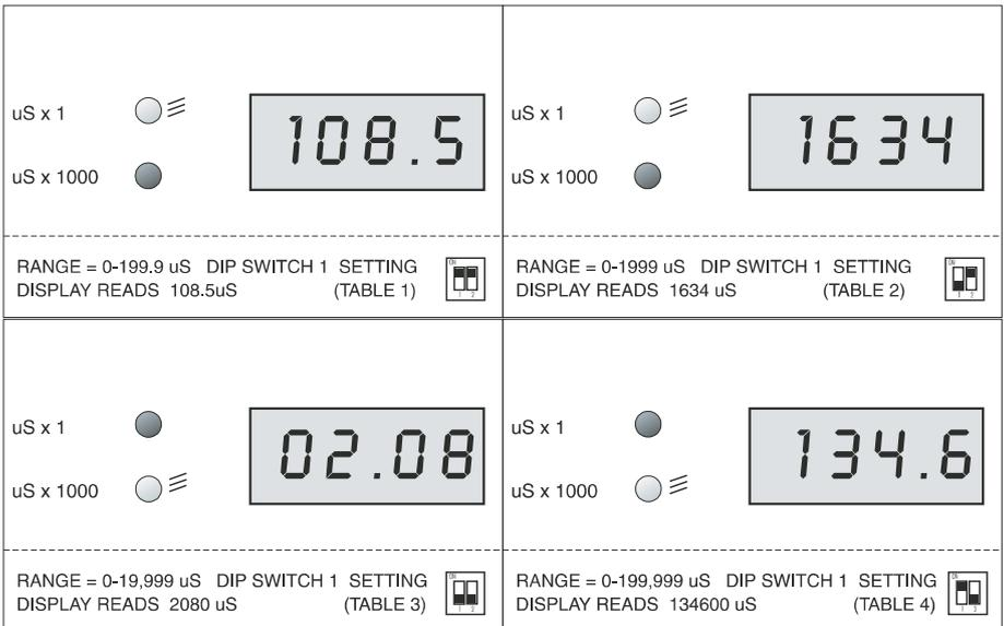
FIG.6 THE DIFFERENT RANGE SETTINGS OF THE DCH-2
