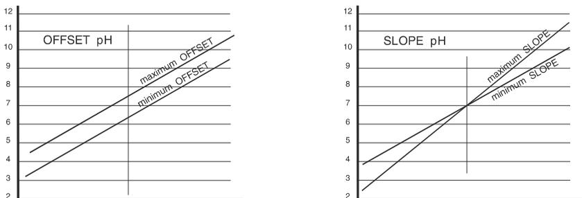
**FIG. 5 THE DIFFERENT EFFECTS OF OFFSET AND SLOPE.**
