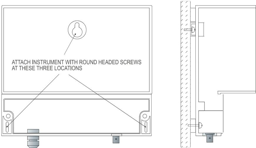
**FIG 3** Attaching the DPH-4 to a wall
