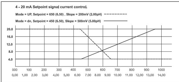
**FIG. 9** 4-20mA Setpoint Signal current control.
