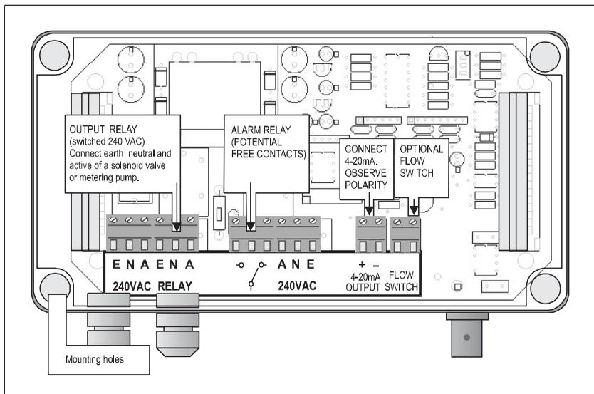
**FIG 5** Terminal layout of the PMV-1.
