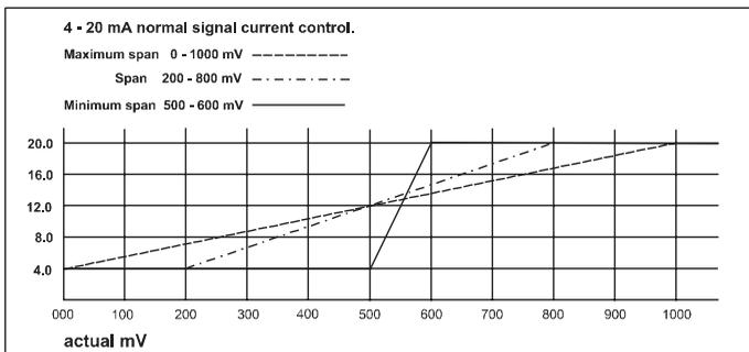
FIG 8 4-20mA normal Signal current control.
