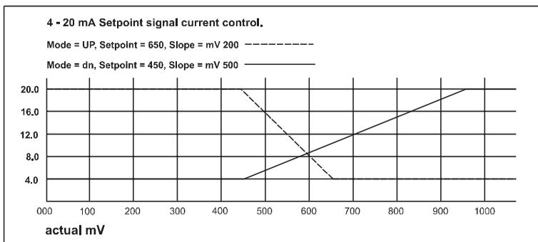
FIG 9 4-20mA Setpoint Signal current control.
