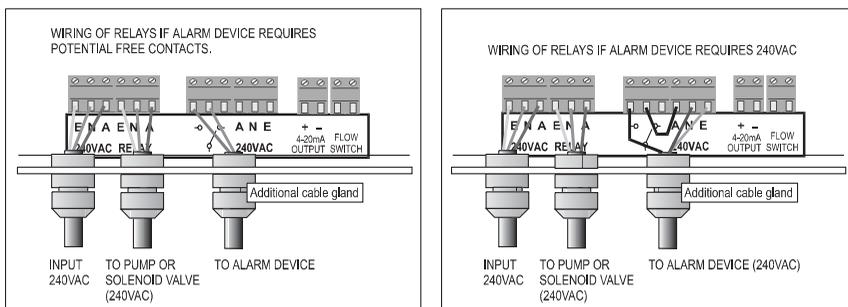
**FIG 4** Wiring examples for the relay outputs.
