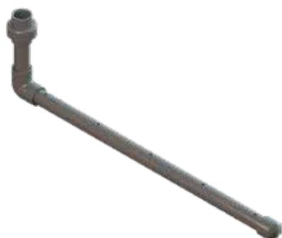
OCDL diffusers allow for two mounting options. Typically, the diffuser would be mounted to a channel wall, parallel to the flow, with the chemical being discharged away from the wall and into the process flow. However with adequate support<sup>4</sup>, the OCDL can also be mounted perpendicular to the flow, spanning the channel, similar to the OCDT. Either configuration can provide a simple, straightforward means of introducing chemical into open channel process flows.
