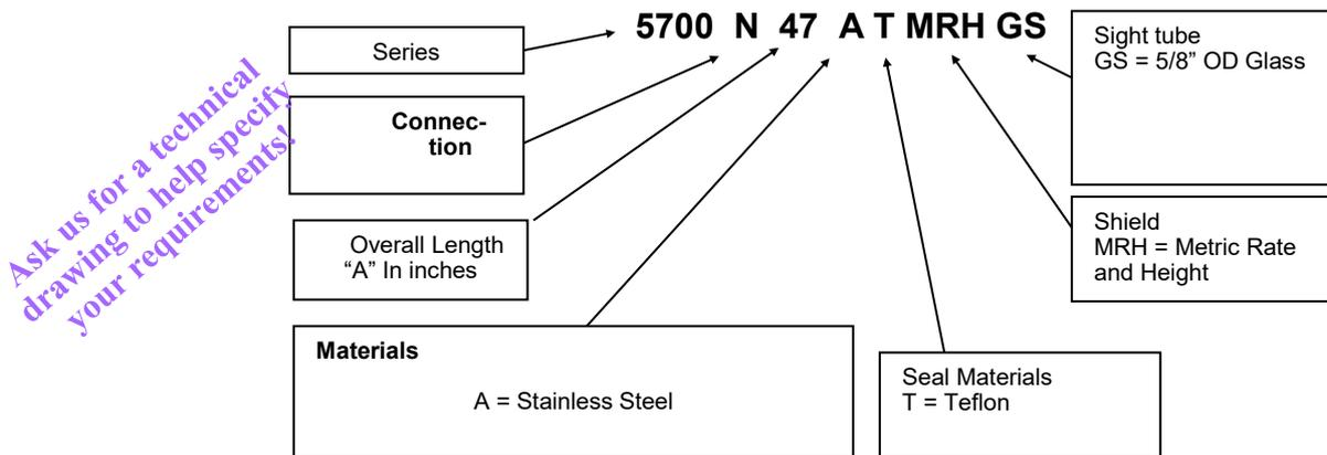
The above part number is for a Series 5700 with 1/2" NPTM of 47" overall length and manufactured from Stainless Steel with Teflon seals, a metric rate and height scale with a 5/8"
