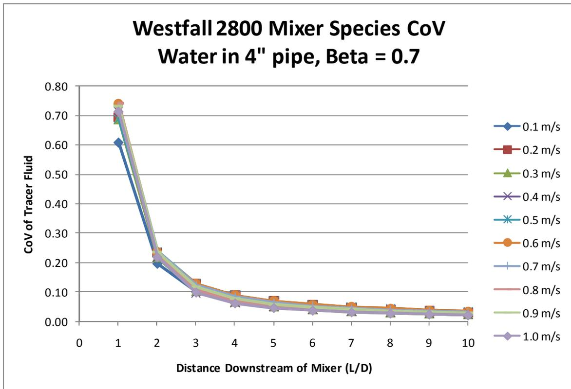
Figure 1: CoV of tracer fluid downstream of mixer.
