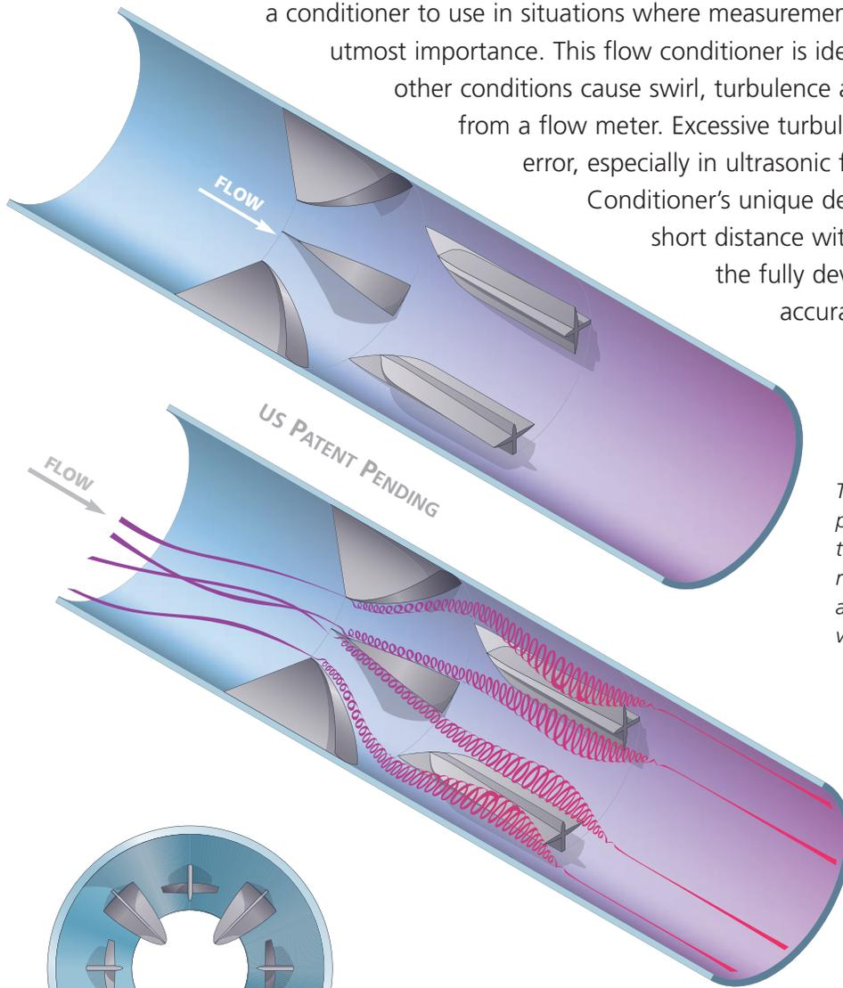
*Two sets of tapered and curved vanes with precisely designed geometry are positioned to eliminate swirl and turbulence without reducing the high velocity core essential to a fully developed velocity profile – all with very little headloss.*
