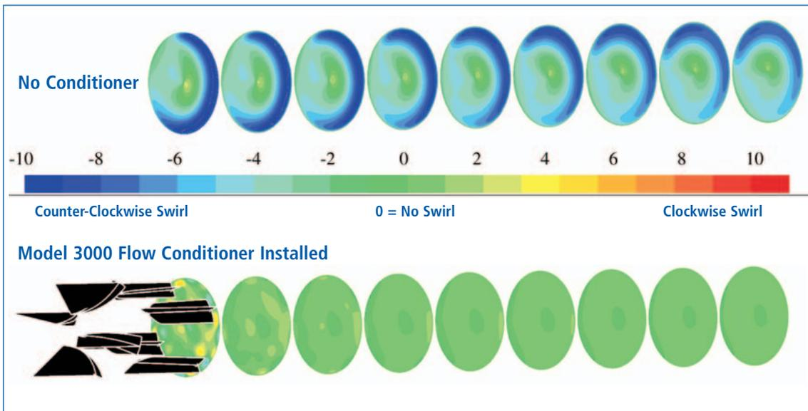
**Model 3000 Flow Conditioner Creates Fully Developed Velocity Profile within Six Diameters**
